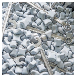
5 Snug-fitting, skin-friendly surfaces thanks to STAHLWILLE's rounded finish
