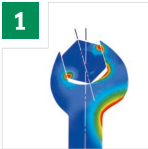
1 Load zones in standard-quality spanners
