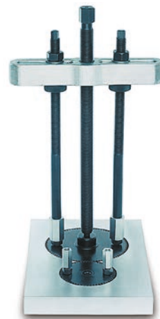
Puller in use for removing gearwheels
